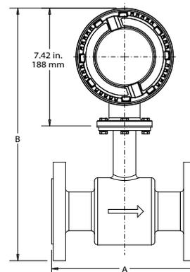
Figure 2: M3000 Remote Mount Junction Box on Detector
